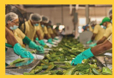
After removal from the plants, the leaves are transported to an on-site processing station where they are washed twice before being filleted by hand. This ensures the rind is fully removed and only the nutritious inner leaf gel is left.
